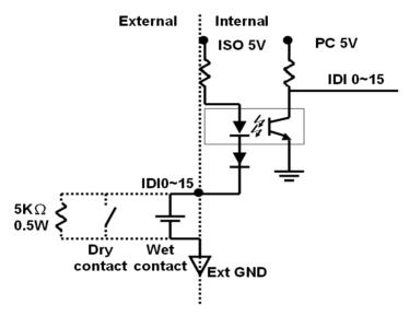
Figure 3.2: Isolated Digital Input Connections
